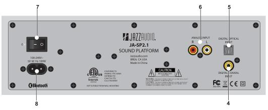
**5. DIGITAL OPTICAL INPUT -** One TOSLINK® connector. Connect to the Digital Optical OUT on a TV or other source. This input is selected by pressing the OPT button on the SOUND PLATFORM IR Remote.
