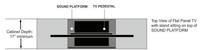
The cabinet top should be at least seventeen inches deep to properly support the SOUND PLATFORM. The SOUND PLATFORM is sixteen and a half inches deep (with grille attached) and extra space will be required between the SOUND PLATFORM and a wall behind the cabinet for cables connecting the SOUND PLATFORM to the TV or other A/V sources (3 inches minimum).
