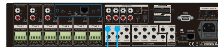
12V DC Trigger for ZONE-1 (for example) to a Motorized Projector Screen
