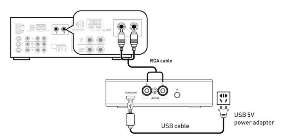
**Step 1** - Use the supplied (d) RCA cable to connect the Subwoofer Pre-Out or LFE output of your AV receiver and to the (a) WSK SUB wireless transmitter Audio Input. You can leave right RCA plug unconnected if you are connecting to a subwoofer as mono signal
