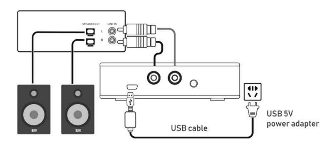
The WSK SUB 5.8G wireless set transmits full frequency audio and can be used for full-frequency active speakers)
