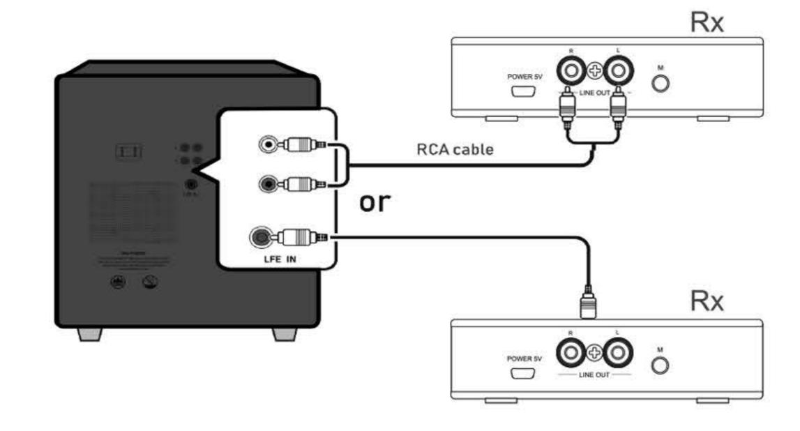
Place the subwoofer at its intended location (refer to your subwoofer owner's manual), and using the supplied (d) RCA cable to connect the (b) WSK SUB wireless receiver audio output to your subwoofer audio input.
