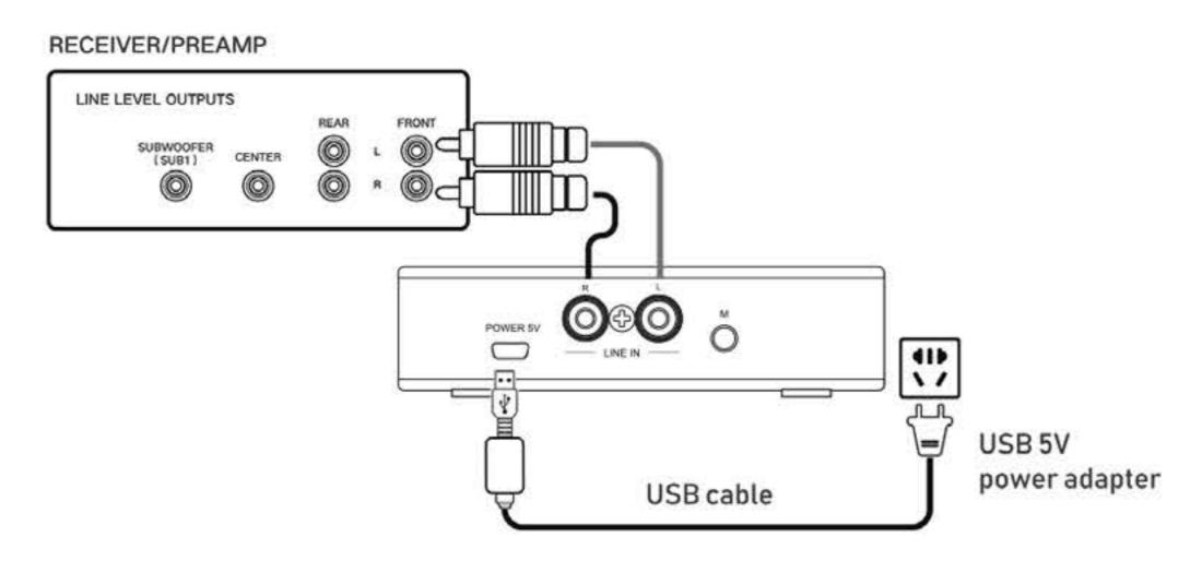
**Step 1** - Use the supplied (d) RCA cable to connector the 2 channel stereo preamplifier's L/R line level Pre-Outs to (a) WSK SUB wireless transmitter L/R input \*Leave right RCA plug unconnected if you have a mono source
