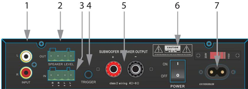
1. **INPUT** - Two, RCA jacks. Stereo or mono audio sensing line level audio input. The SMP200 will turn ON when a line level audio signal is present on either jack. Amp will turn OFF after 15 minutes of no audio signal.
