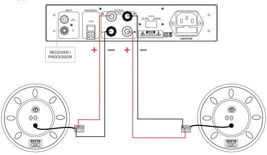
NOTE: The above example shows 5 total speakers. Using the 10W selection, you will need an amplifier with at least (5) x (10) = 50W. A good rule of thumb to remember is that the total number of speakers multiplied by the setting you select, cannot exceed the output power of the 70V/100V amplifiers. You should select an amplifier with 20% greater power; in this case, an amplifier that delivers about 60W.
