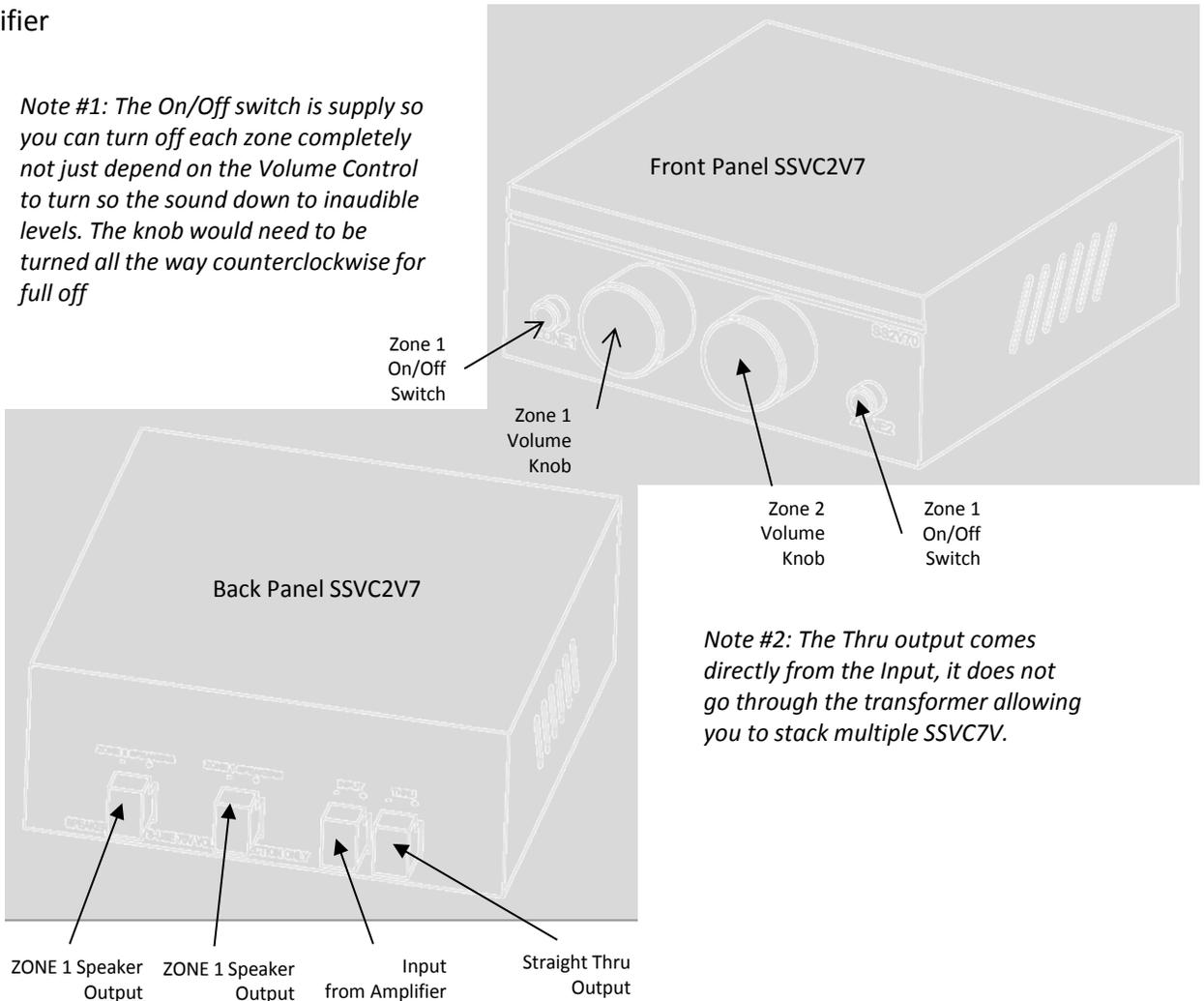
*Note #2: The Thru output comes directly from the Input, it does not go through the transformer allowing you to stack multiple SSVC7V.*
